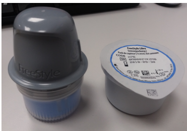
Figure 3: Unboxing: the sensor comes in 2 parts. On the left, the gray applicator contains the electronic board. On the right, we have the enzyme sensor in a sterile package
